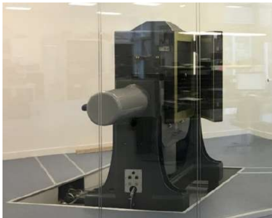
Figure 6. Picture of (left) a double axes rate table and (right) its associated frames and axes.
